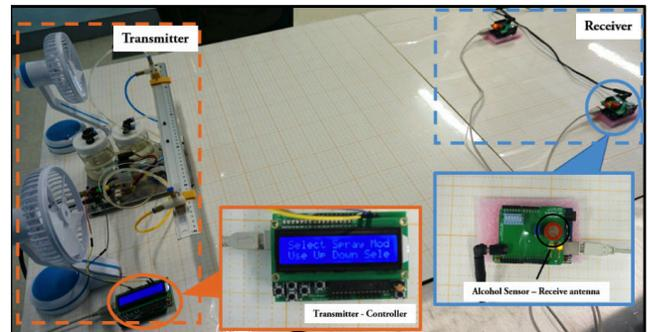
Figure 1: The tabletop molecular MIMO communication platform.
